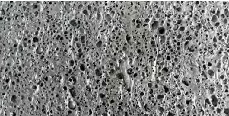
AL-FG-12.7-SM-1S (small cells, open one side), detail
