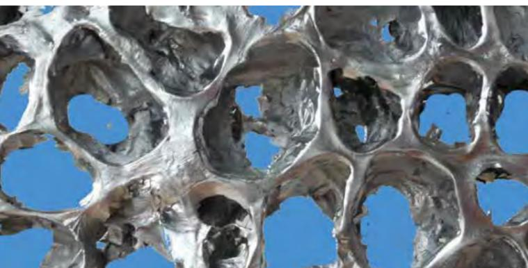
AL-FG-12.7-LG-2S (large cells, open both sides), detail
