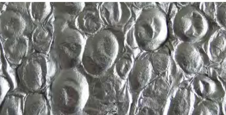
AL-FG-12.7-LG (large cells, both sides closed), detail
