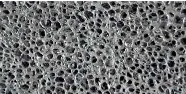
AL-FG-12.7-MD-1S (medium cells, open one side), detail
