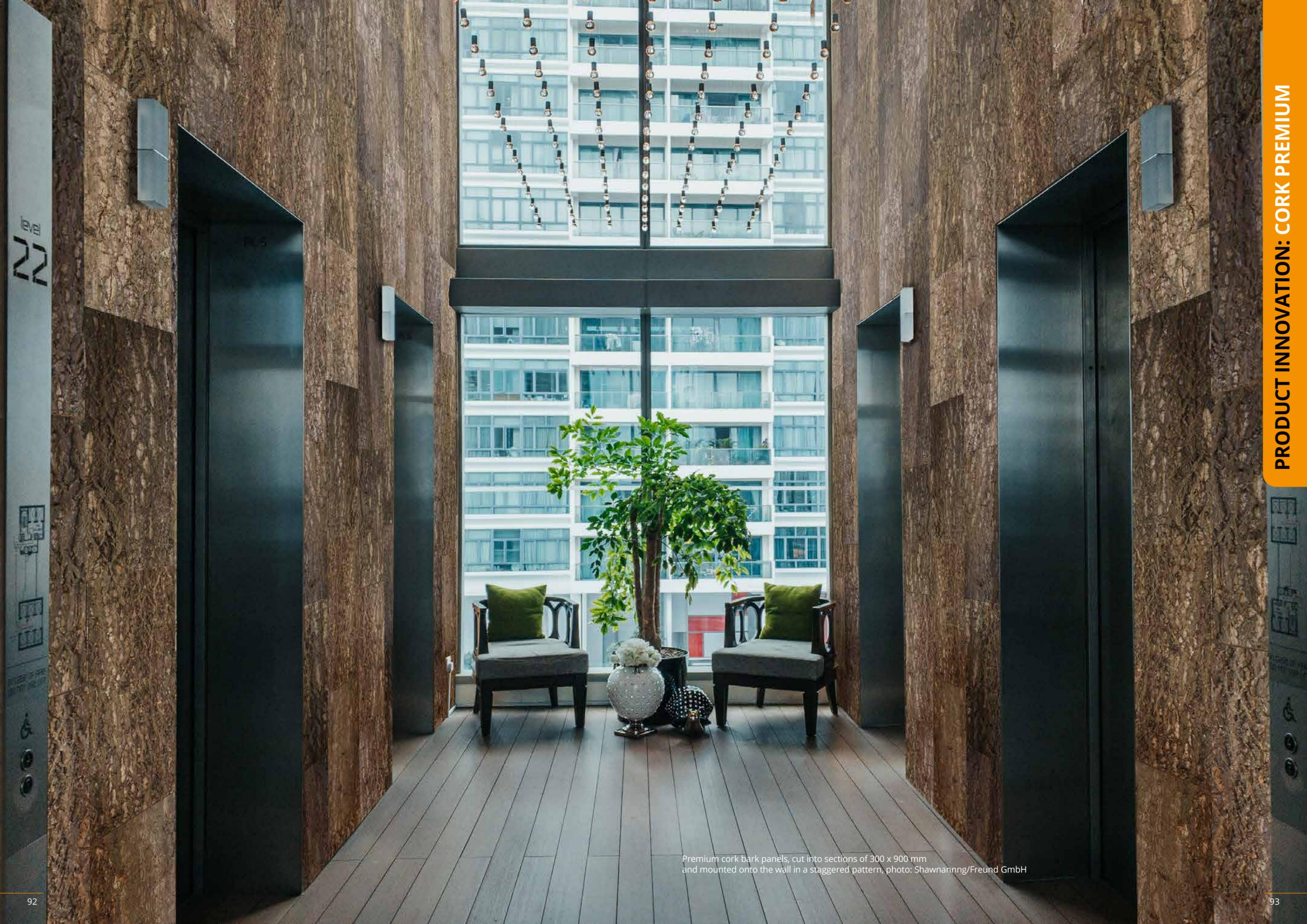
Premium cork bark panels, cut into sections of 300 x 900 mm and mounted onto the wall in a staggered pattern, photo: Shawnanng/Freund GmbH
