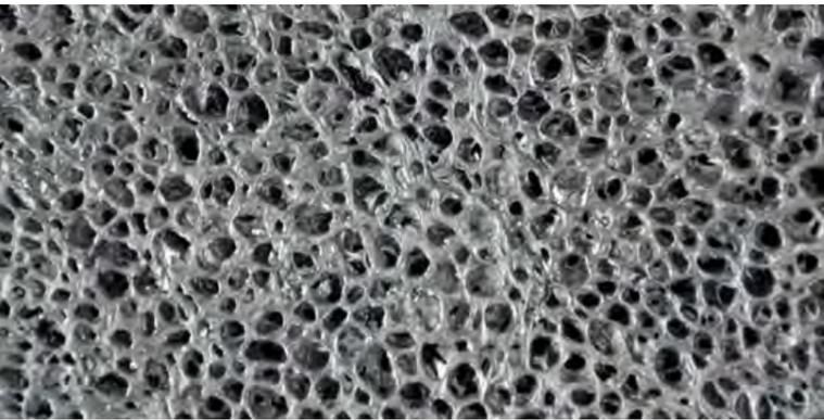
AL-FG-12.7-MD-1S (medium cells, open one side), detail
