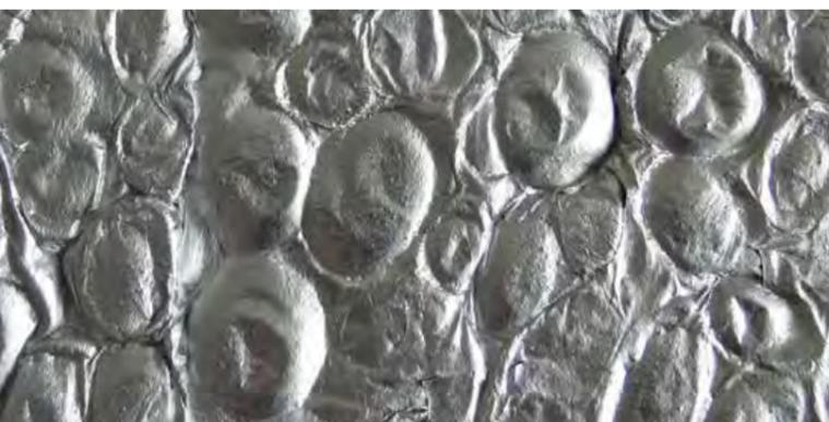
AL-FG-12.7-LG (large cells, both sides closed), detail
